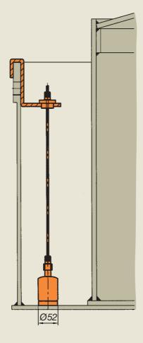
The transducer is suitable for installation into a central control system. As a complete alarm system, the optical acoustic alarm transmitter is available for the sginal processing of one (OAA1) or two (OAA2) level sensors. So the optional signal processing of the overfill safety alarm and the leakage alarm can be done..
